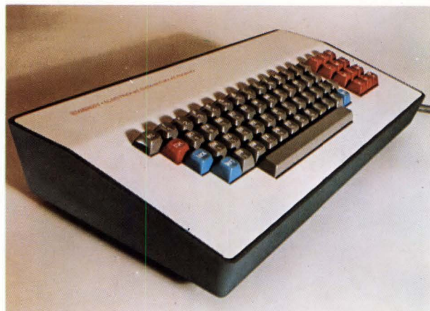
Standard ASCII Tri-Mode mechanical keyboard. (Cherry)
