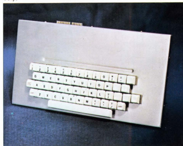
Contactless capacitive keyboard has illuminated keycaps (Raytheon)
