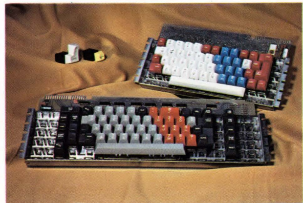
Hall effect solid state keyboards feature MOS encoding. (Micro Switch)
